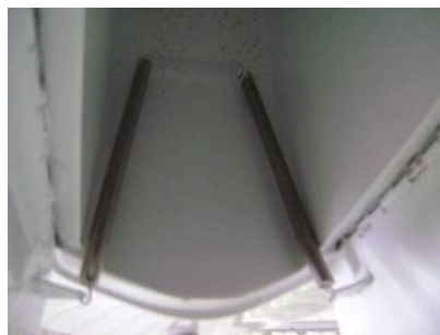
b) Springs inside the nose gear doors.
