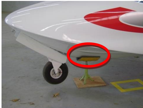
(a) Support under the keel
