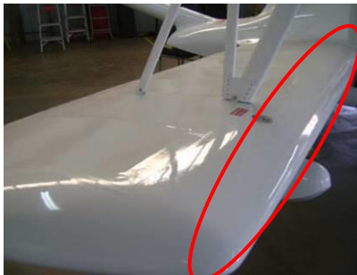
(a) Fuel Tank
