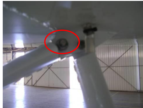
b) Main strut attachment with upper wing
