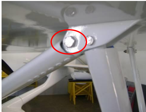
b) Main strut attachment with upper wing
