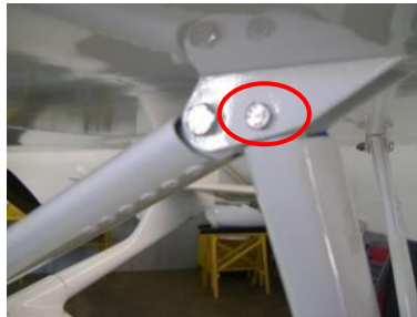
c) Inner strut attachment with upper wing
