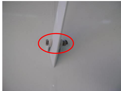
d) Inner strut attachment with lower wing
