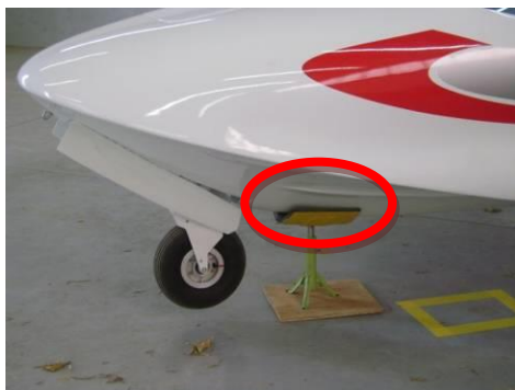
(a) Support under the keel
