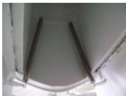
b) Springs inside the nose gear doors.
