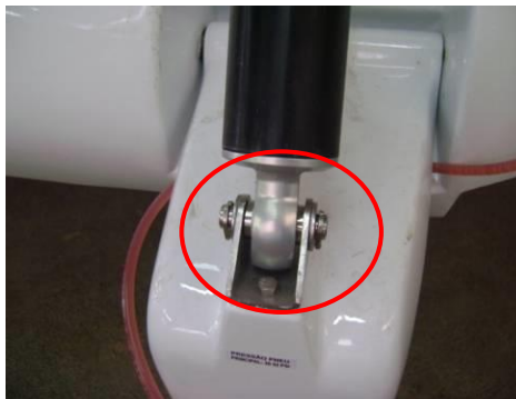
a) Attachment with the main gear leg
