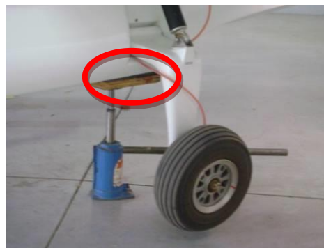
(b) Jack under the main gear
