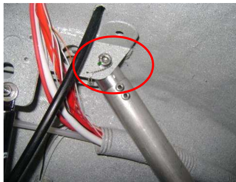
b) Attachment inside the fuselage
