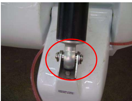
a) Attachment with the main gear leg
